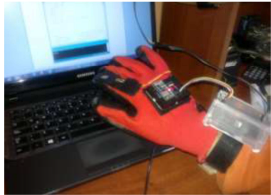
Figure 6. Prototype of the inertial capture system for computer access of the disabled
